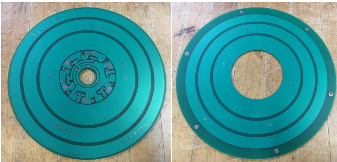
Figure 2-5: Initial three-phase capacitive power coupler prototype rotor (left) and one of two stator disks (right).
