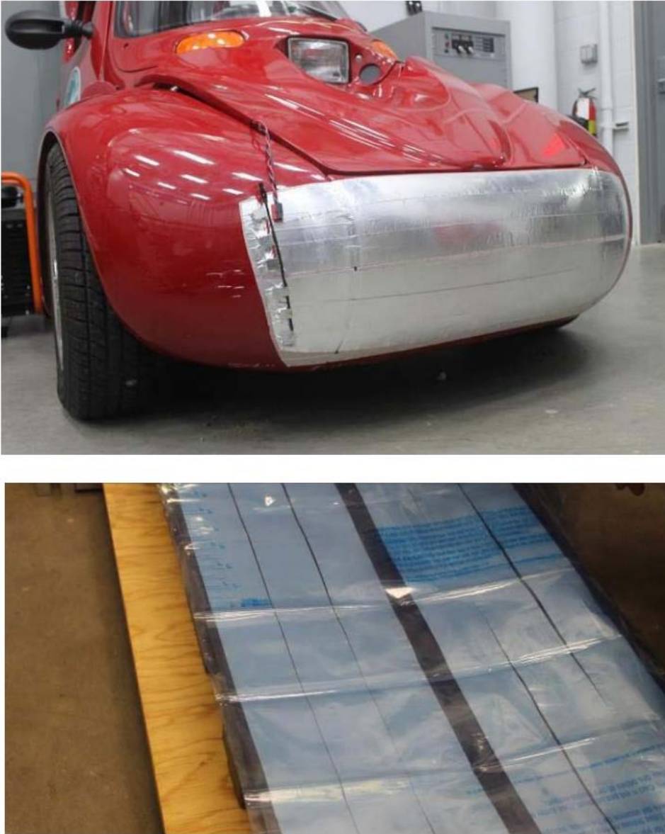
Figure 1-13: Conformal bumper electric vehicle CPT structure showing receiving electrodes on bumper (top) and wall mounted conformal electrode structure (bottom) [58].
