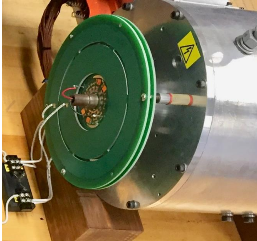
Figure 4-4: CPC assembly mounted on WFSM end bell.
