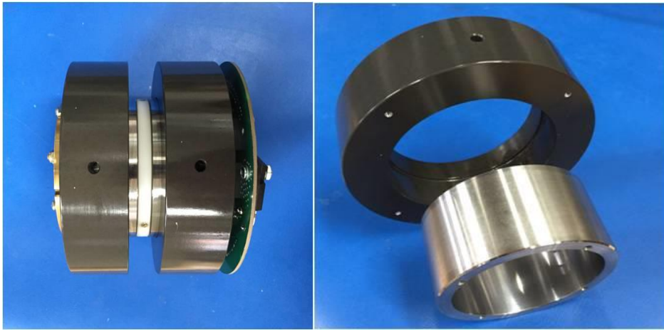
Figure 1-17: Hydrodynamically levitated journal bearing capacitive power coupler. Assembled with rotating rectifier board (left) and individual bearing and shafting components (right) [2].
