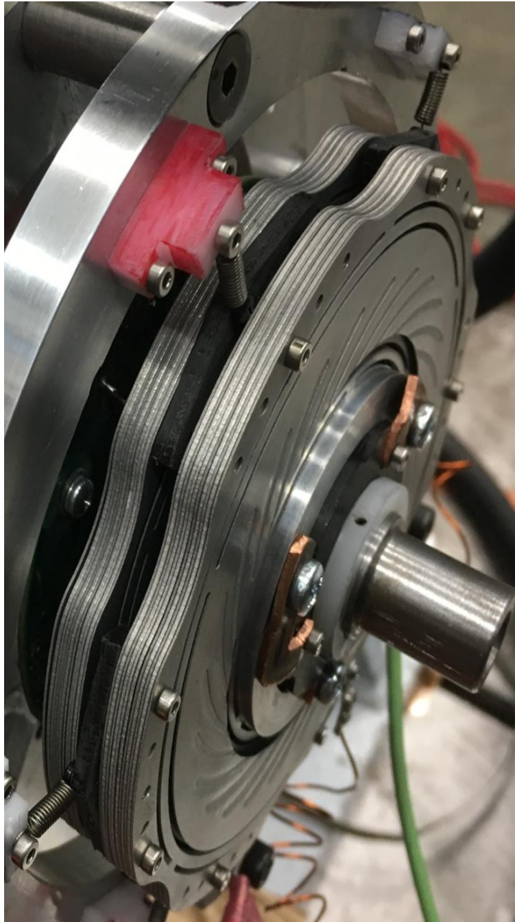
Figure 1-19: Aerodynamically levitated “hydroflex” axial thrust air bearing used as capacitor electrode structure in a 1kW CPT system for WFSM field excitation [62], [63].
