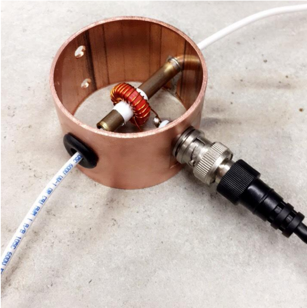
Figure 3-2: Current sensing transformer of simple construction used for closed loop frequency control for soft switching.
