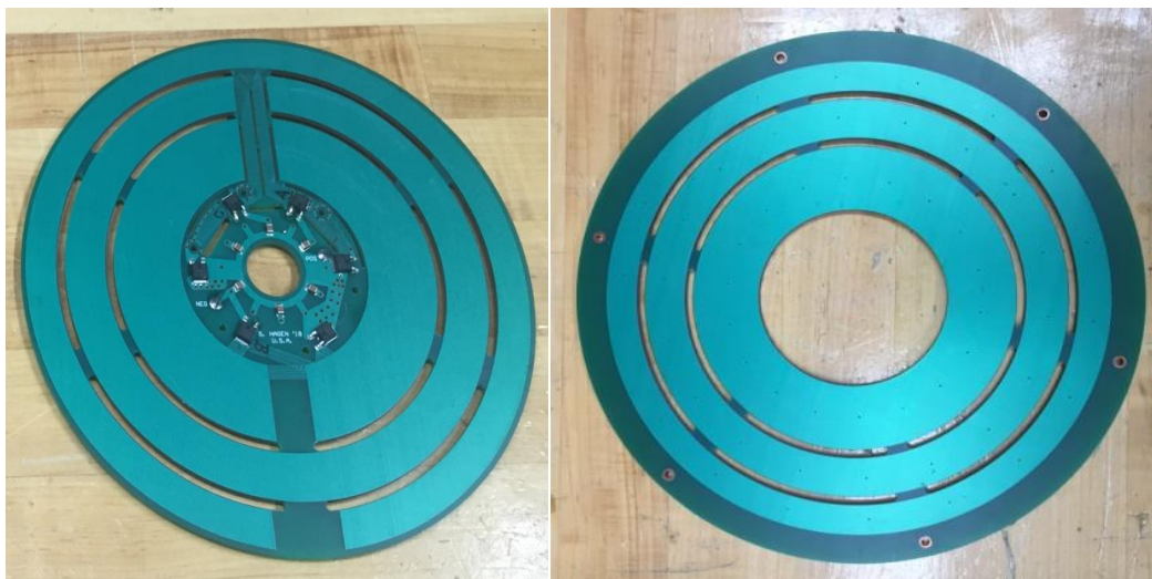
Figure 2-11: Improved 3-phase prototype with slotting and elimination of trace overlap.
