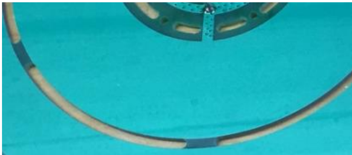
Figure 2-7: Close-up photograph of “slotting” between capacitor electrodes. Also seen is the slotting between the inner electrode and the rotor electronics section.
