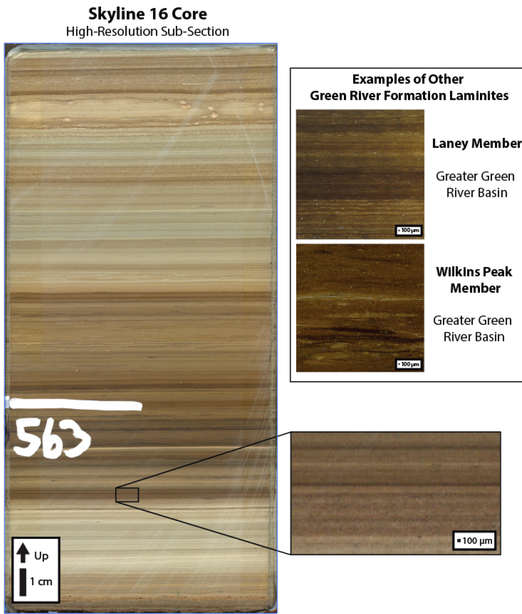
Figure 3: Laminated mudstone in the “Upper R-6” zone of the Parachute Creek Member of the Green River Formation captured in the Skyline 16 core. This interval was studied using the 100 micrometer capabilities of the Avaatech XRF core scanner and the 25 micrometer resolution capabilities of the Bruker M4 micro-XRF. Included for comparison are examples of laminites from the Laney Member (Arco Washakie Basin 1 Drill Core: Section 17 T14N R99W) and Wilkins Peak Members (Breathing Gulch Site: 41° 48.50' N, 109° 17.64' W) of the Green River Formation in Greater Green River Basin of Wyoming.
