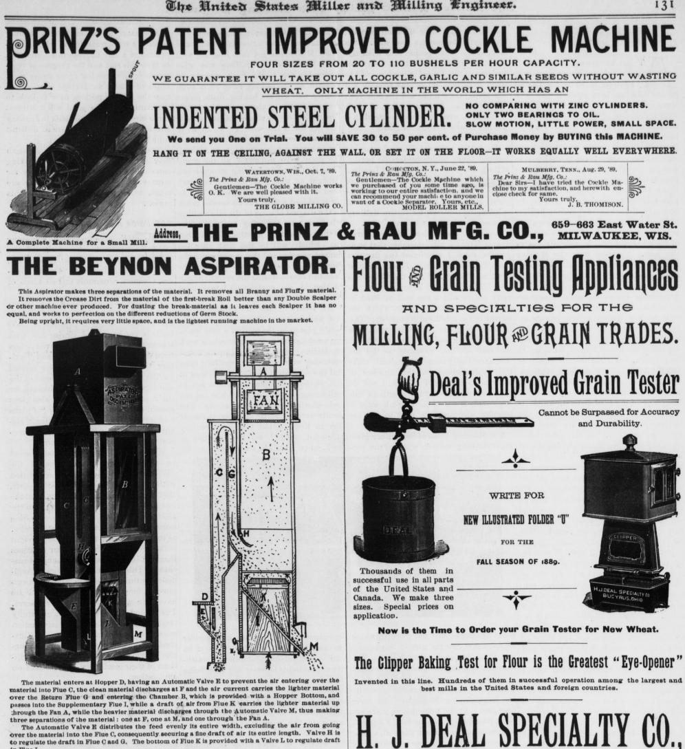
The Automatic Valve E distributes the feed evenly its entire width, excluding the air from going over the material into the Flue C, consequently securing a fine draft of air its entire length. Valve H is to regulate the draft in Flue C and G. The bottom of Flue K is provided with a Valve L to regulate draft in Flue I.
