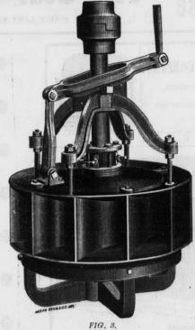
Fig. 3 shows the wheel complete, ready for shipment or to be set in a flume. The fourarmed spider or bridge-tree attached to the bottom of the outer case has in its center the wooden step prepared by a special process of the manufacturers.
