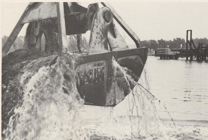
A dredge in Green Bay harbor. Sediments constantly fill port areas and navigation interests seek deeper channels to accommodate larger and larger ships. Most ports in Wisconsin and elsewhere have toxic materials locked in bottom sediments that require expensive, special handling. When tests show PCBs or heavy metals like lead, chromium or mercury in dredge spoil, the material must be isolated in diked disposal areas enclosed by clay and rock levees to permanently confine the pollutants.
