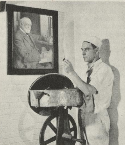
The original Babcock tester provided an accurate measurement of the butter-fat content of milk—and helped make dairying a major industry. It was invented by Professor Stephen M. Babcock, whose portrait is seen here.
