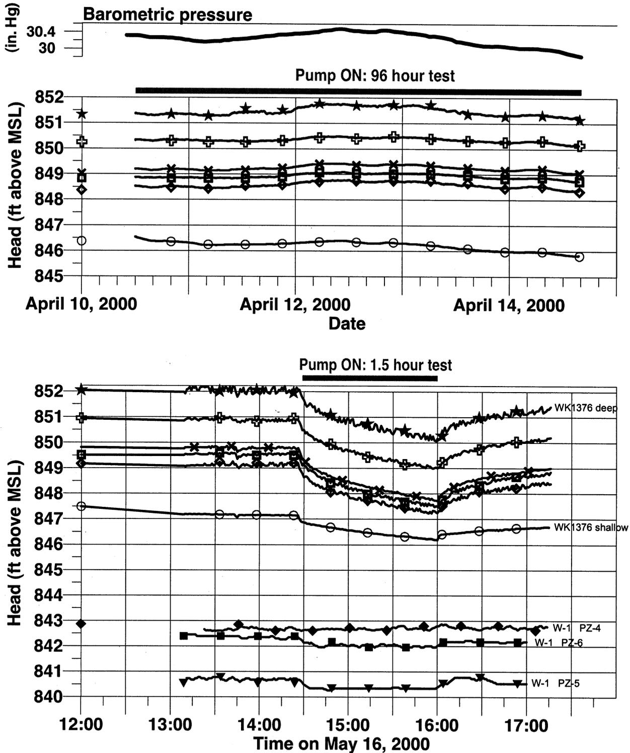
**Figure 15:** Selected observation well heads during deep aquifer (top) and shallow aquifer (bottom) testing. Symbols correspond to intervals located in Figure 1. No significant head change was observed in monitoring points not shown.
