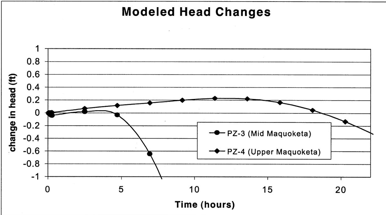
**Figure 6b:** Modeled head changes in the Maquoketa and Sinnipee formations due to a step decrease in the Sinnipee Group Dolomite. Head change not shown for PZ-1 at this scale.
