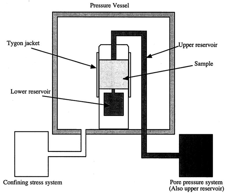
**Figure 2:** Diagram of the pulse decay apparatus.
