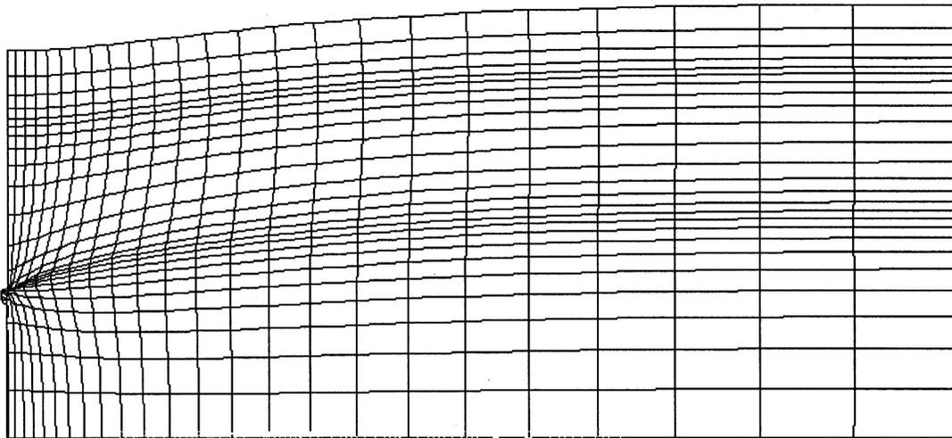
**Figure 5:** Deformed finite element mesh at 16 hours. Displacement exaggerated  $2.5 \times 10^5$  times.
