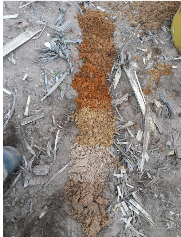
(Left) Examples of cores collected from each field using the Geoprobe®. Cores provide good ability to understand the soil profile. Sample can be saved and analyzed at a later date.
