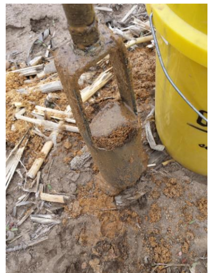
(Left) Contracted services for use of Geoprobe®. With the water table at ~10-12 feet contractors were able to collect samples from 20 locations per day.
