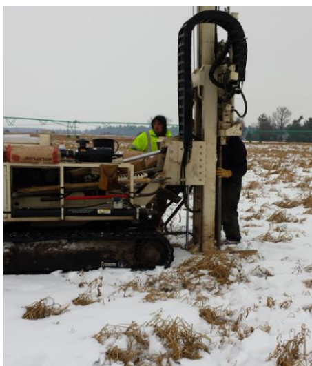
(Left) Contracted services for use of Geoprobe®. With the water table at ~10-12 feet contractors were able to collect samples from 20 locations per day.
