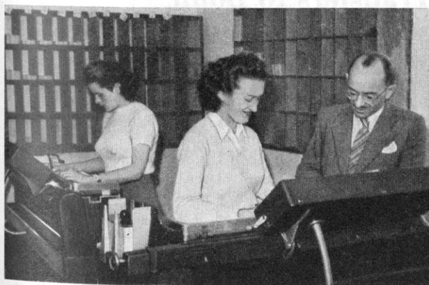
Answers are punched onto IBM cards, then run through sorting machines. Results are percentaged, analyzed.
