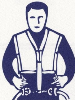
Step 3 After you leave the plane, inflate vest by pulling sharply on the two cords at bottom.
