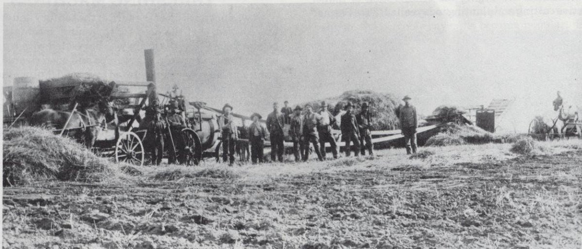
Circa 1900 Straw burner steam engine used for power to operate the threshing machine owned by Eggebrecht & Hamann Company. Straw on the wagon was used as fuel to fire the steam engine. The engine was pulled by horses. Straw was moved on the threshing machine on an elevator as it had no straw blower.
