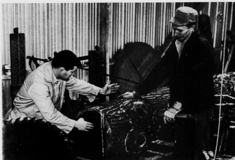
Grade sawing can produce lumber worth $15 to $30 more per thousand board feet as compared with old-fashioned sawing methods.
