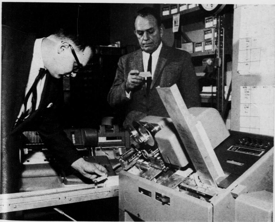
Here's the machine that makes the plastic registration cards supplied to boat owners. It can turn out about 1,200 cards a day.
