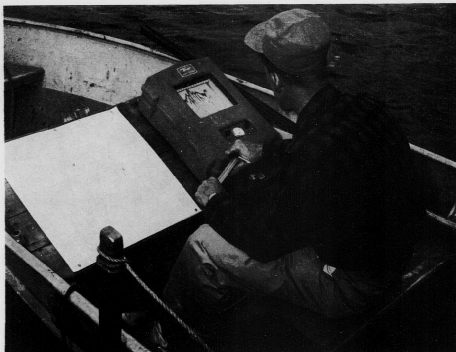
Sonar equipment speeds up the gathering of data for lake contour maps. Such maps, sold by map companies, are in great demand by fishermen.
