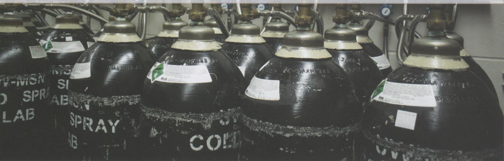
Rows of pressurized nitrogen gas canisters that are used in the acceleration of metal powder through the barrel of the cold spray device.
