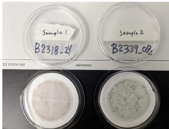
Figure 33: Photograph of vacuum filtered solid residue from acidic digest of post-corrosion salt pills.
