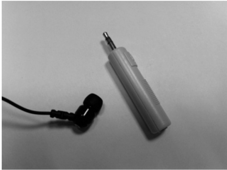
Figure 2.2. NR microphone in the ear and attenuator at the end of the cable
