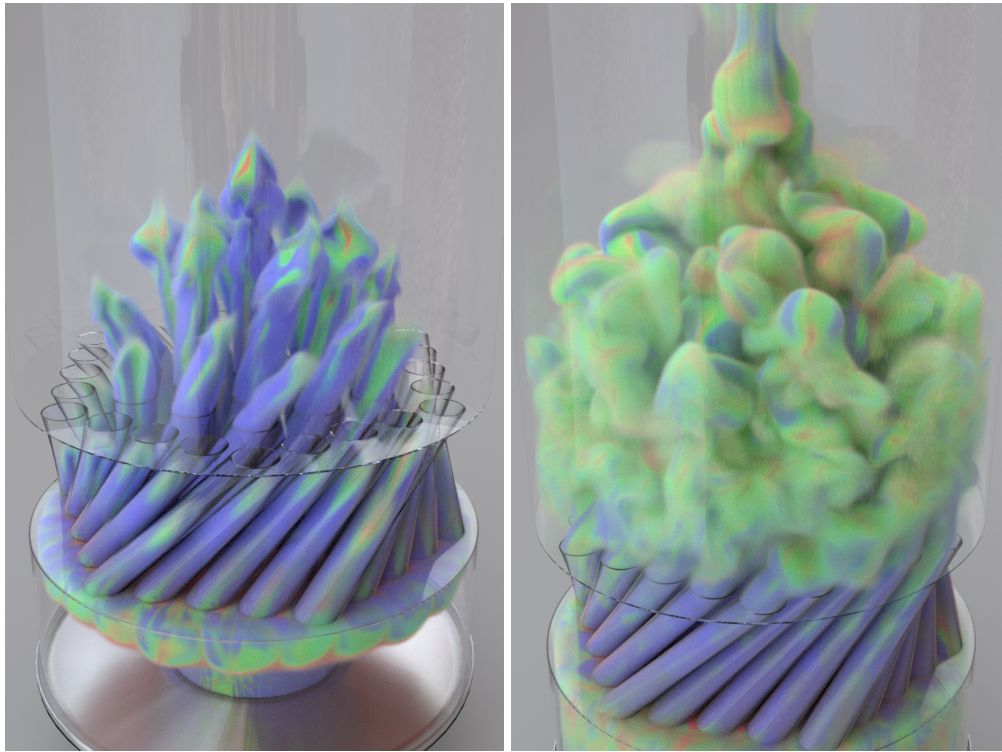
Figure 3.3: Smoke injected from the bottom of a cylinder, and forced through a twisted bundle of cylindrical holes. Color corresponds to vorticity magnitude. Total 1.2B active cells, in a 1024^2 \times 2048 grid.
