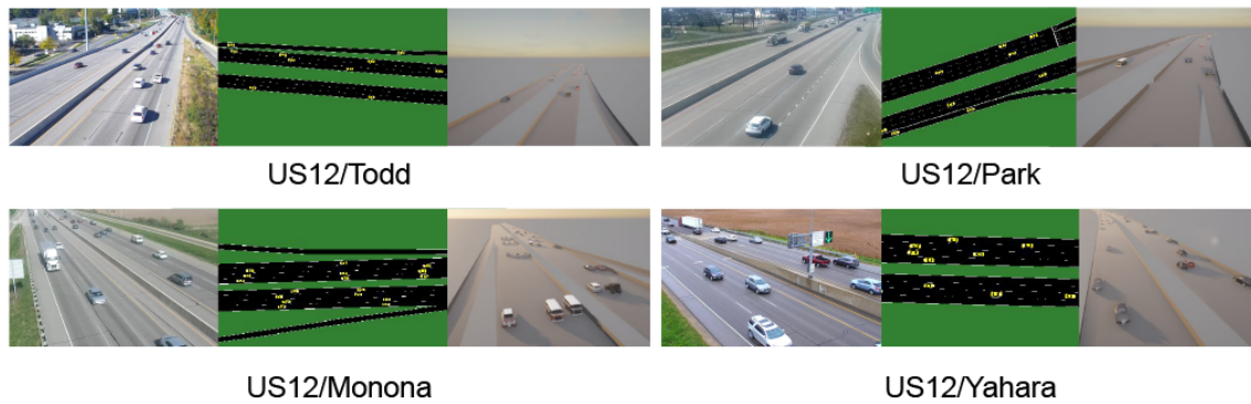
Figure 2.10: Digital twin synchronization with SUMO and CARLA at multiple locations, driven by real-time empirical vehicle trajectories.
