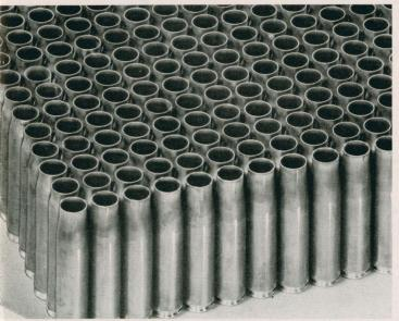
Rigid process control is necessary in the drawing, annealing and machining operations of cartridge case manufacturing in order to hold the close tolerances required.
