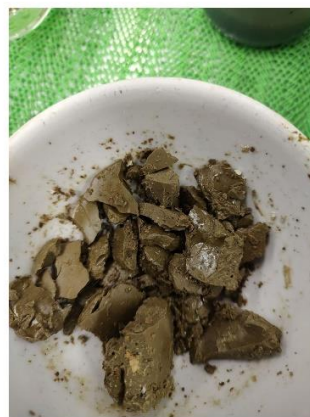
Figure 5.13. Scale up issues observed at high catalyst loadings. Top: THF and product separation of products obtained in 75 mL Parr reactors. Middle: Changes in product composition by decreasing catalyst loading (50 to 15g of catalyst). Bottom: Particle and product behavior at high catalyst loadings (50g) on a hotplate.
