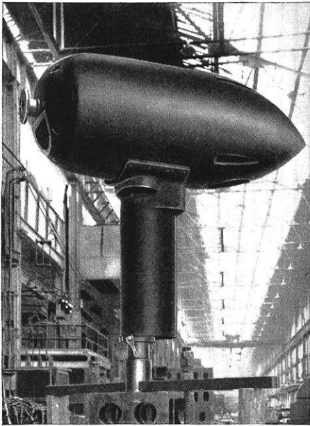
—Courtesy General Electric Company. Induction motor used to test airplane propellers.
