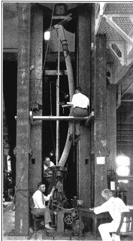
Test of a laminated wood arch in the large testing machine at the Forest Products Laboratory.
