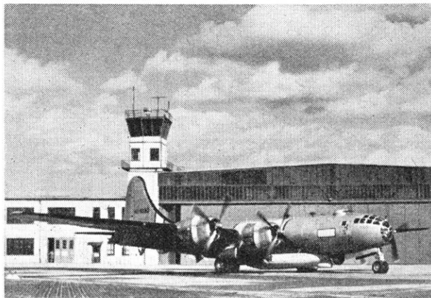
Pictured is one of four SB-29's, aerial search and rescue version of the Superfortress, on arrival at Wiesbaden Air Base. The planes are equipped with radar equipment and lifeboats. The main item, the A 3 lifeboat, is 30 feet long and can be dropped from 1,400 feet and remain upright. Its engine carries up to 200 gallons of gasoline and can be started and guided by radio. (USAFE photo)
