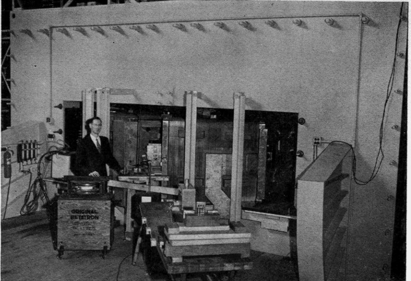
DONALD W. KERST, '34, (above) now a physicist at the University of Illinois, has built the world's biggest betatron, a 300 million volt radiation machine which accelerates electrons to enormously high speeds so they may be used to split the nuclei of atoms. Unlike smaller, earlier models (and Kerst also built the world's first in 1940) this new betatron will be used exclusively for nuclear research.
