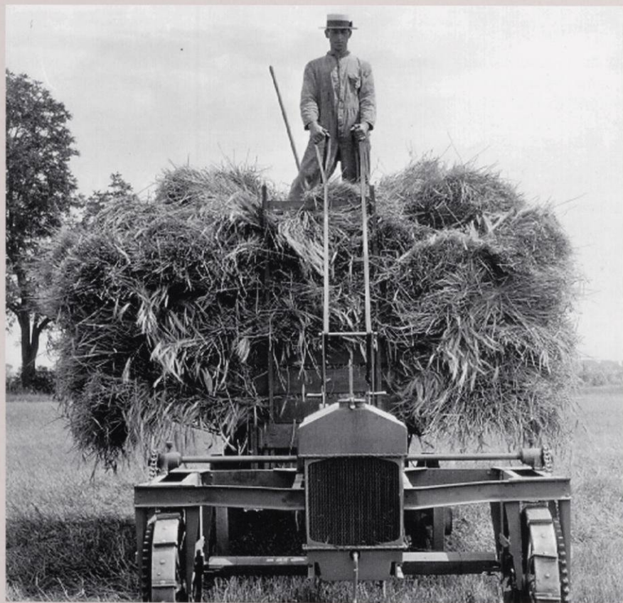
Above: Samson Tractor's Model D, the 'Iron Horse,' was steered by reins. The quirky design was an attempt to attract farmers used to handling teams of horses.
