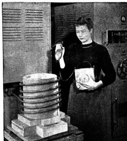
Norma L. Gullberg, A.B., Chemistry, Clark University '46, takes a reading with an optical pyrometer on a high temperature furnace used for catalyst support tests.
