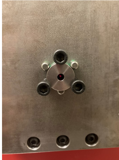
Figure 3.17: A front view of the 5 mm tungsten aperture. The aperture is held with the pins that have been press fit into the steel plate and the screws which can be removed to switch out the apertures. This picture was taken after alignment during a measurement course so the 1 m green laser can be seen at the back plane of the aperture at the POM and the cross laser can be seen shining through the aperture.
