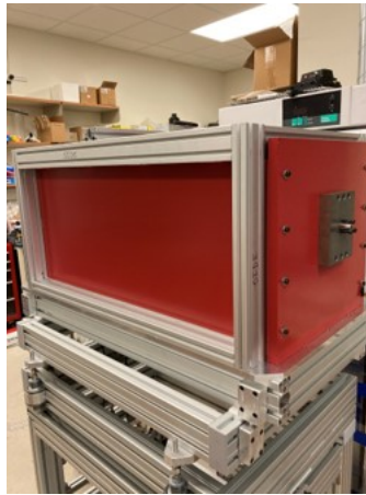
Figure 3.12: Assembled shielding for the FAC standing on the FAC cart.
