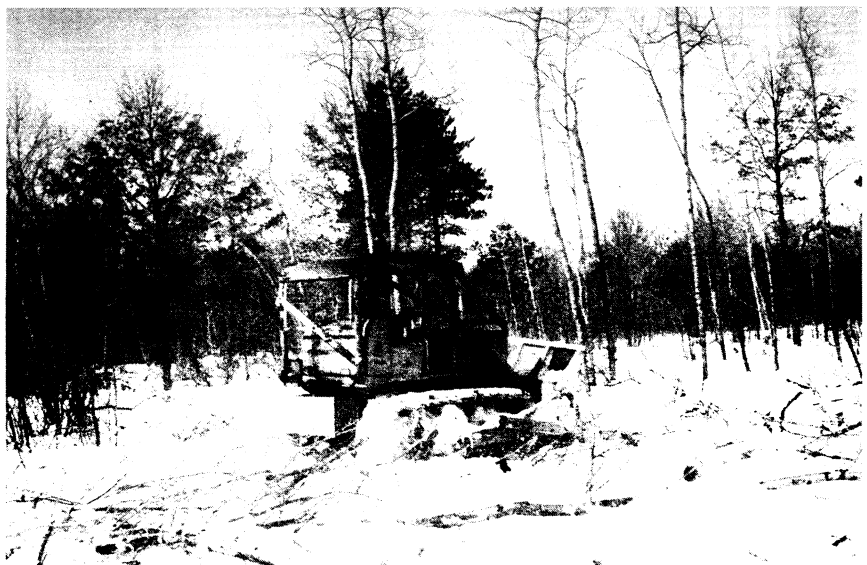
Shearing was conducted using KG blades or chain saws to achieve a complete clear cut following timber sales in aspen stands.
