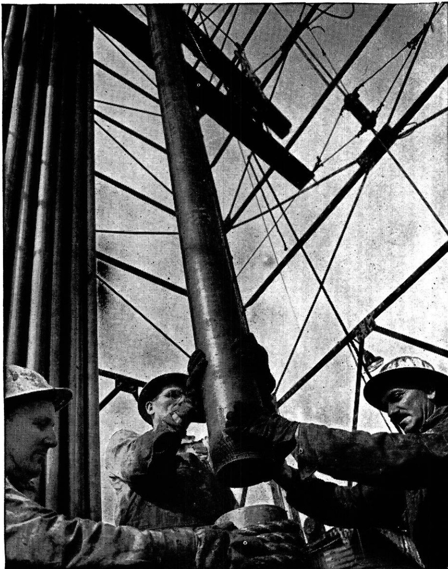
Lengths of Republic Electric Weld Casing are rapidly joined together and lowered hundreds or thousands of feet into an oil or gas well to line it with tough steel—to protect its walls against the tremendous pressures that otherwise might cause collapse of the hole.
