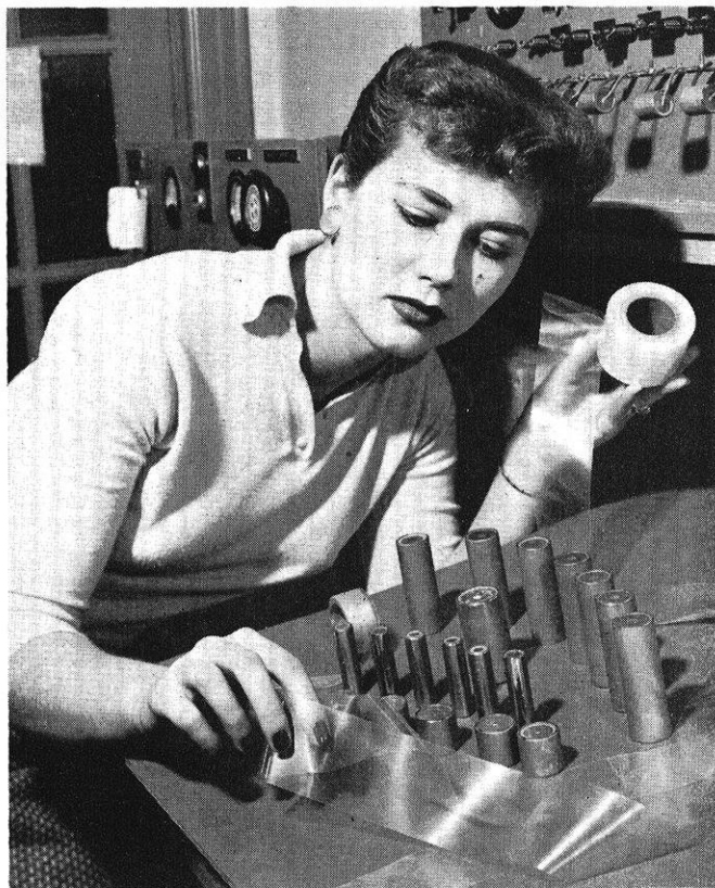
This ribbon-like irradiated polyethylene tape is used to wrap coils for sintered-plate batteries, nickel-cadmium type. Hand-wrapped around the battery cores, irradiated polyethylene tape forms a stable chemical-resistant insulation between core and cylinder.
