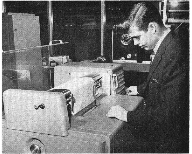
The High Speed Printer of the Remington Rand Univac System for handling large volume output. It is capable of printing 600 lines a minute.
