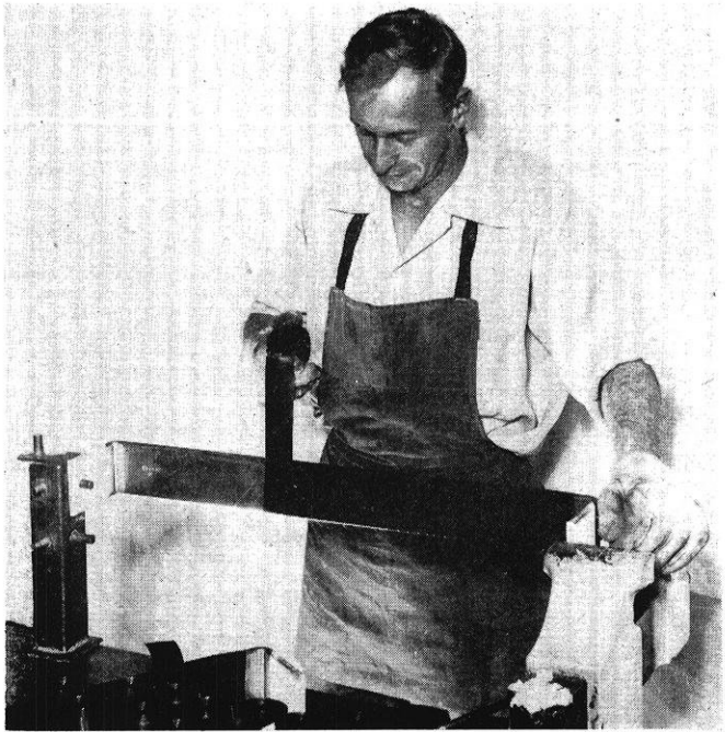
Irradiated polyethylene tape is hand-wrapped on bus bar for metal-clad switchgear. The tape forms a tight, uniform insulation, free of voids or bunching, while the number of wraps per voltage level is reduced about 50 per cent.
