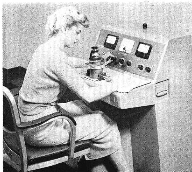
The new G.E. X-ray Microscope, adapted for direct-viewing.
