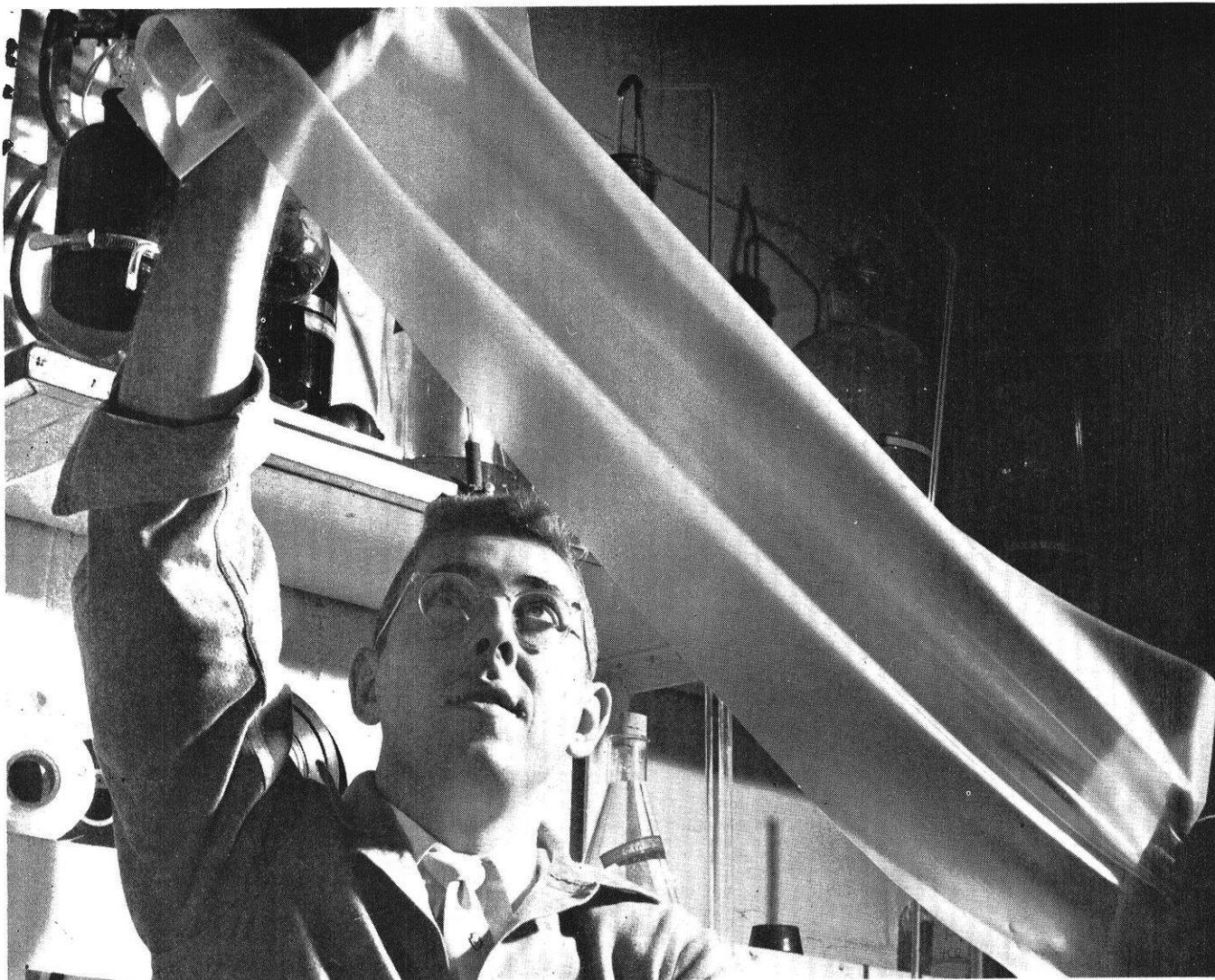
A technician gives roll of irradiated polyethylene preliminary check for uniformity. Starting out as conventional polyethylene, the irradiated tape is bombarded with high-velocity electrons to make it flexible and resistant to chemicals, moisture, heat and stress.
