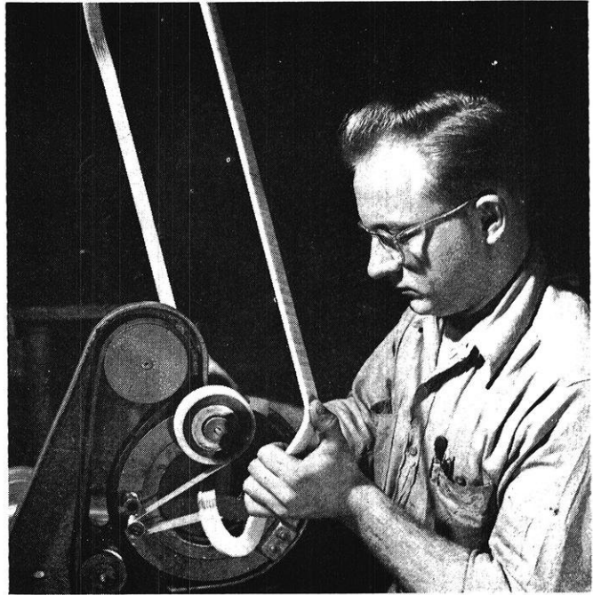
This machine "wraps" 600 complete laps of insulating tape per minute on a generator coil. Irradiated polyethylene tape is wrapped around bends and knuckles of the three-turn coil, then heat-bonded to provide a tight seal against moisture, dust, and dirt.
