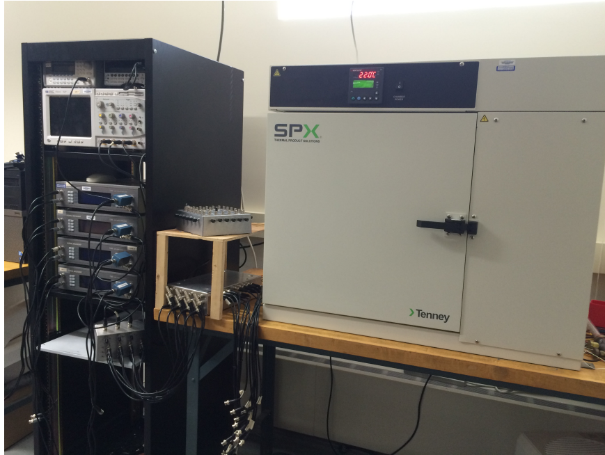
Figure 4.5: Picture of the 3\omega experimental setup. The large box on the right, labeled SPX, is the Tenney Junior Compact Temperature Test Chamber. On the left, an instrument rack houses an Agilent 33250A waveform generator, an HP Infinium oscilloscope, and four Signal Recovery 7265 lock-in amplifiers. The three homemade electrical boxes between the instruments and sample chamber allow for electrical breakout, switching, and house a series of unity gain operational amplifier circuits.
