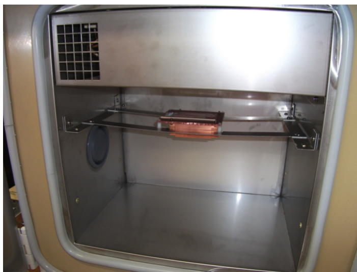
Figure 4.8: Interior of the Tenney Junior chamber, including the shelf and sample stage, both made in house. There are two sets of mounting brackets, upper and lower. In this picture the shelf is mounted in the upper brackets.
