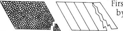
The polycrystalline diamond blank microfractures because of its structure. Natural cleavage planes of mined diamond (right) cause it to break off in larger pieces.
