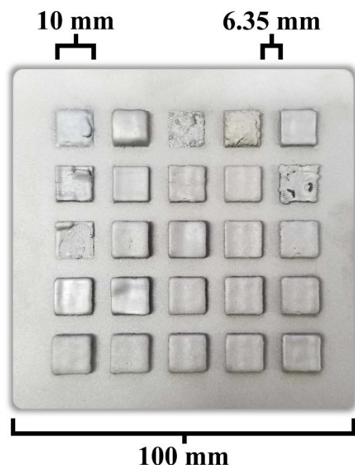
Figure 36: Photograph of the as-built Cr-Fe-Mn-Ni array printed on a 316-stainless-steel build plate after media blasting to remove adhered powders. Prior to any machining, sample heights and surface finish as printed vary as a function of composition.
