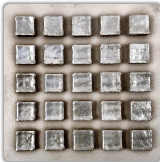
Figure 23: Compositional array produced by in situ alloying via additive manufacturing (AM). For reference, each square stub is 1 cm 2 while the build plate is 10 cm on a side.
