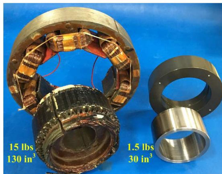
Figure 1.19. A comparison of a traditional brushless exciter with a capacitive brushless exciter [36]
