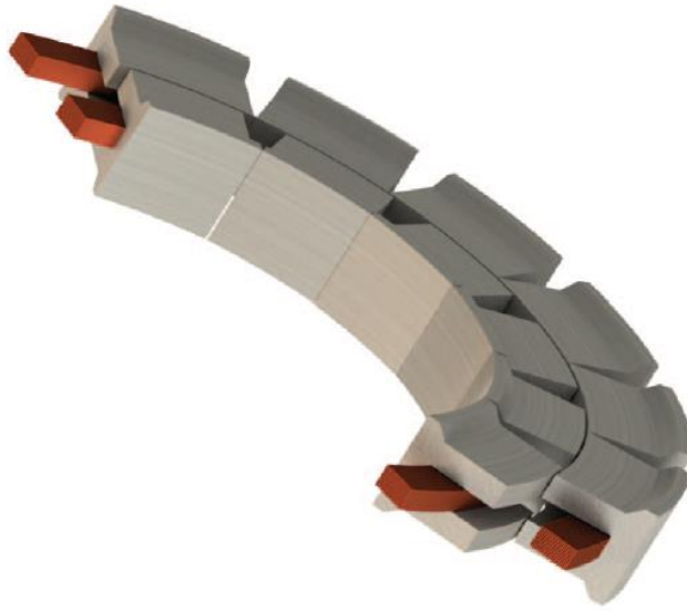
Figure 1.26. Concentric RT made by radially oriented electric steel [47]
