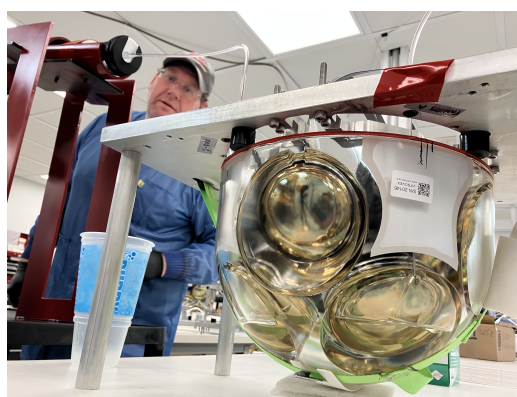
Figure D.23: A view of the pads mid-way through backfilling. The white cutout observed protects the vessel from gel dripped accidentally, and is peeled off after backfilling
