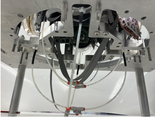
Figure D.18: The bladders are connected with T-junctions during inflation with epoxy, which prevents loss of compressive pressure in case of leaks developing in the bladder
