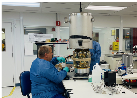
Figure D.26: A. Arbuckle of PSL operating the pressure chamber to flush the LOM atmosphere with nitrogen.
