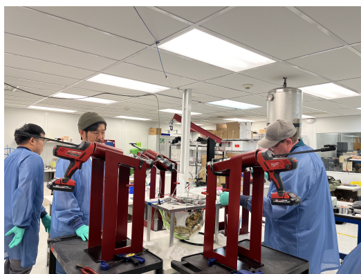
Figure D.22: With the prototype jig used for the Upgrade module production, we are able to fill four pads simultaneously.
