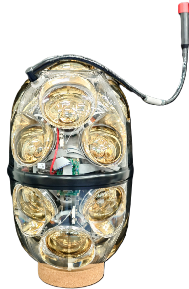
Figure 11.5: The 18 PMT Long Optical Module (LOM) design. Picture courtesy N. Shimizu
