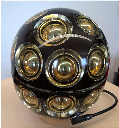
Figure 11.2: The multi-PMT Digital Optical Module (mDOM). Picture courtesy L. Classen
