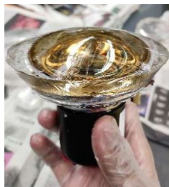
Figure D.7: Plastic gel 'shells' to be filled with liquid gel in-situ. Figure D.8: A gel pad coupled to a PMT
