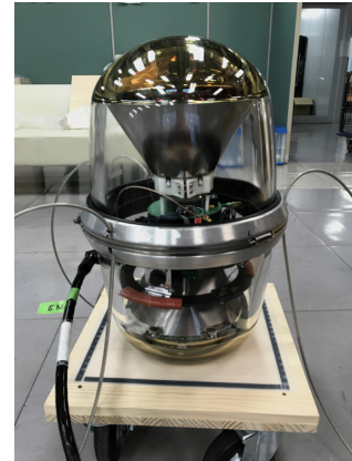
Figure 11.3: The D-Egg, an acronym for Dual optical sensors in an Ellipsoid Glass for Gen2. Picture courtesy N. Shimizu
