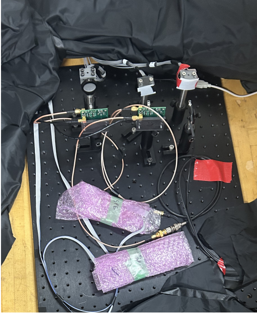
Figure D.43: The Flasher LEDs used for injecting pulses for PMT testing. There are two Flasher 2 boards used for generating the LED signal, and sending a trigger signal to the timing wuBases in the lower half of the image, to register as waveforms. The leftmost board is used for dim SPE signal studies, with the ground glass diffuser between the LED and the optical fibers. The centre board is used for bright narrow pulses, as part of the tests of the low gain channel readout. This board is connected to a separate timing base, and also sends a trigger signal to a function generator. This function generator is used to generate bright wide and double pulses, injected into the PMTs using the LED on the right
