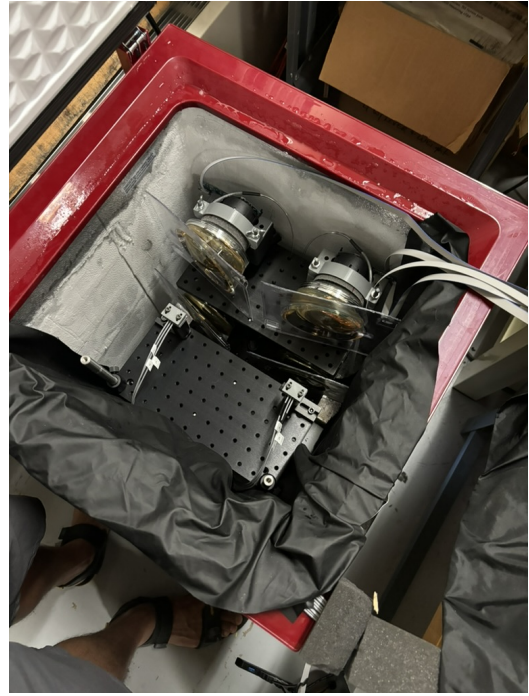
Figure D.44: A view of the PMT test-bench in the freezer dark box, with three optic fibers mounted in front of each PMT. These fibers bring in the photon signal from the three sources visible in Fig. D.43
