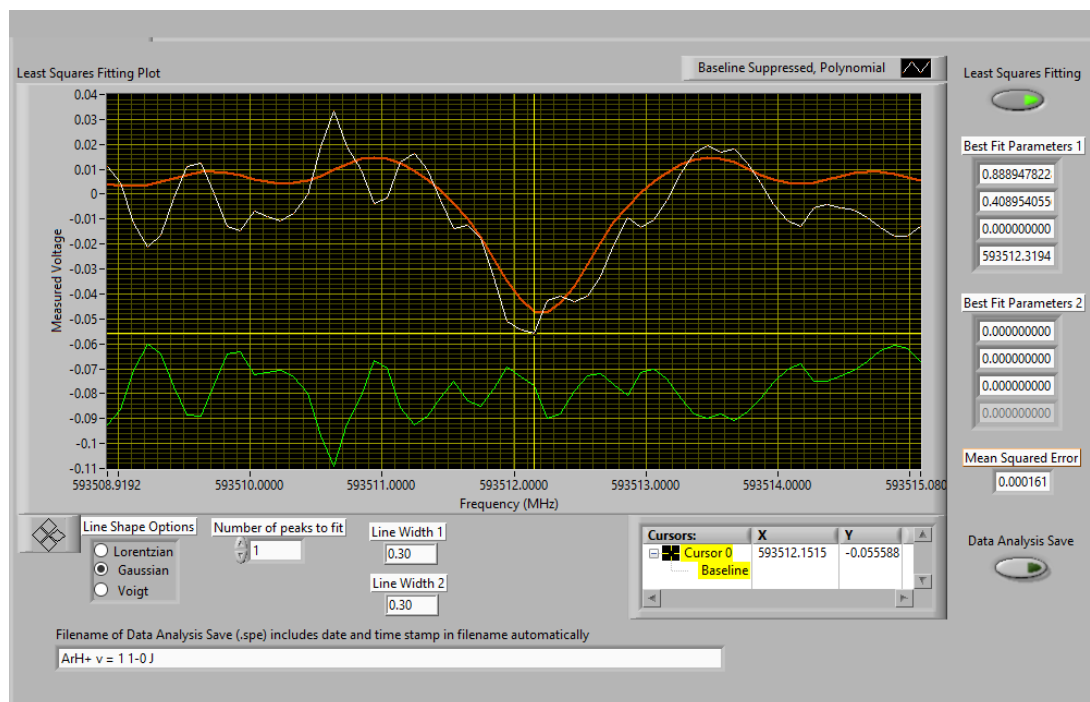
Fig. B.2. ArH + first vibrationally excited-state rotational transition from J = 0 to J = 1 observed at 593512.15 MHz.
