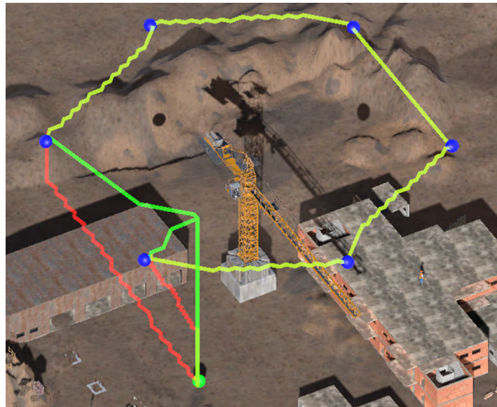
Figure 31. Visualization of planned drone paths with (green) and without (red) soft cost consideration in Scene A. (Yellow line is two lines overlapping)
