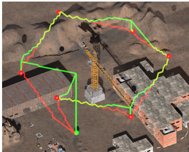
Figure 32. Visualization of planned drone paths with (green) and without (red) soft cost consideration in Scene B. (Yellow line is two lines overlapping)
