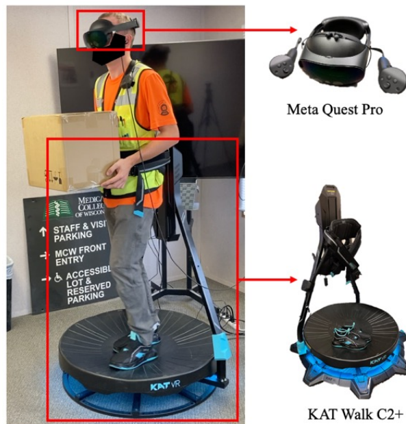
Figure 2. Test participant wearing a Meta Quest Pro VR headset on KAT Walk C2+
