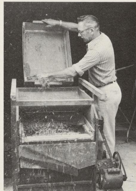
A homemade winnowing machine separates the grain from the chaff.
