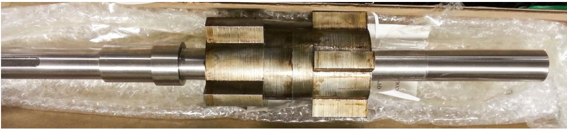
Figure 8.2. Fabricated rotor of the proof-of-concept dual-stator 6/4 FSPM machine.
