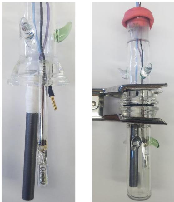
). The use of a reference electrode means that this set-up must be used with a potentiostat rather than a power source.
