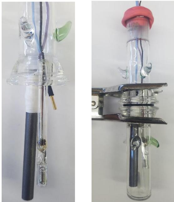
Increase the stir rate until good convection is observed. Connect the potentiostat leads to the electrolysis cell electrodes, taking care to make sure the correct leads are connected to the correct electrodes and that the leads are not contacting any other conductive materials. Standard connections for all Pine potentiostats are described below:
