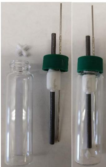
**Figure A.1.** Electrochemical bulk electrolysis cell used by students.
