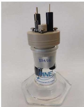
**Figure B.9.** Pine Research cell setup for electrochemical analysis.
