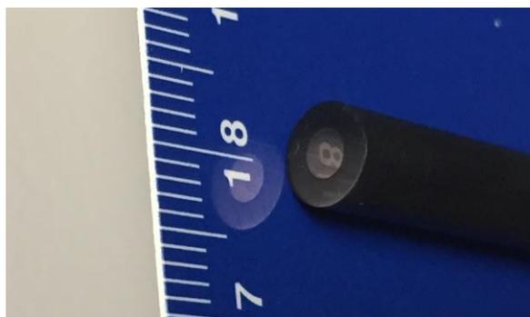
**Figure B.1.** Demonstration of shiny surface of polished glassy carbon (GC) electrode
