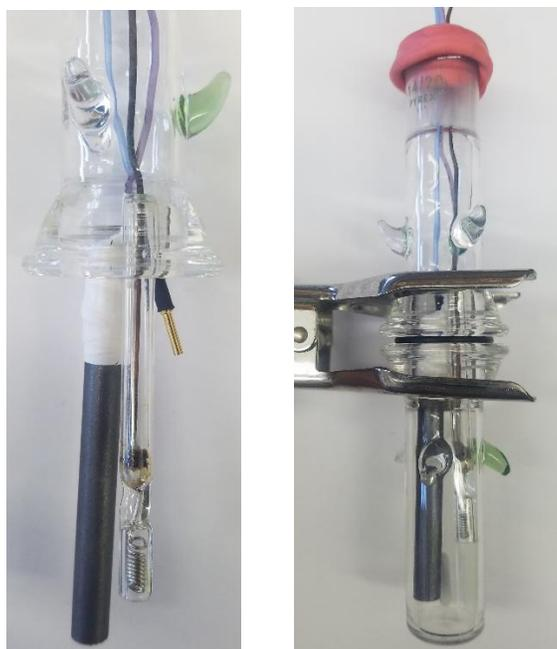
**Figure A.2.** Example of alternative electrochemical bulk electrolysis cell used by instructors during lab development.
