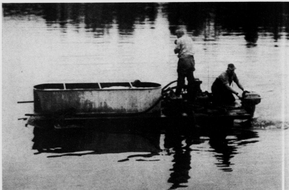
Equipment such as this is used to distribute toxicant, where it is feasible to destroy stunted fish or undesirable species and then re-stock.
