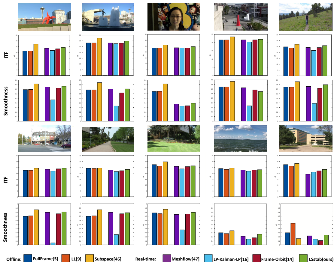
Figure 5.11: Comparison with state-of-the-art video stabilization algorithms. Higher ITF and Smoothness means better stabilization result.
