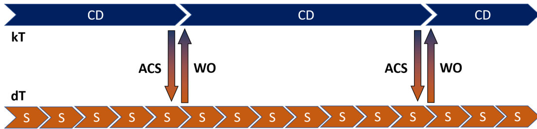
Figure 4.2: Two-thread asynchronous contact detection collaboration pattern, where the dynamics thread advances the physics continuously while the kinematics thread occasionally waits for updated state information to commence an ACS update.
