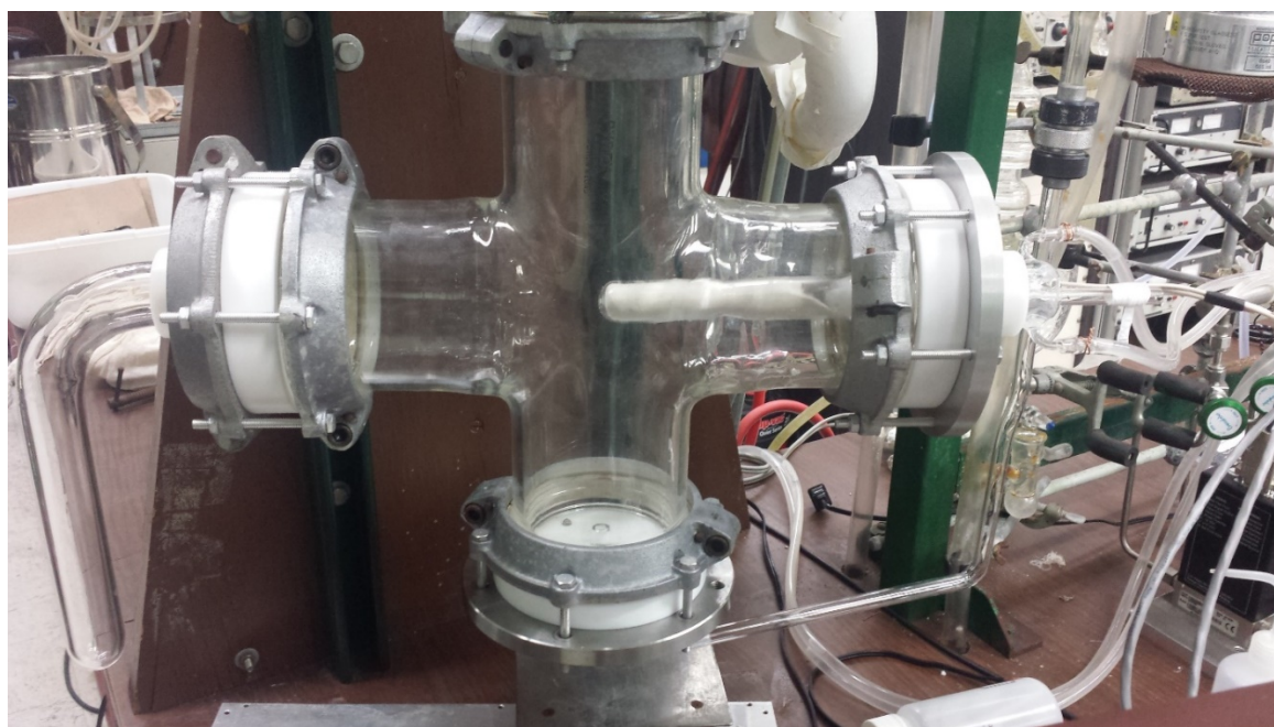
Figure 3.8 A Pyrex cross added to the spectrometer to give new ports for a pyrolysis heater (right) and a thick-walled glass piece that can be used to condense sample (left).
