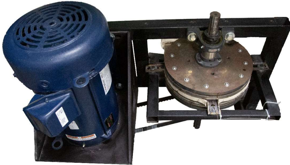
Figure 4-1: An example of the 12-Pole Double-Array Disc-Type PMIP studied in this work.
