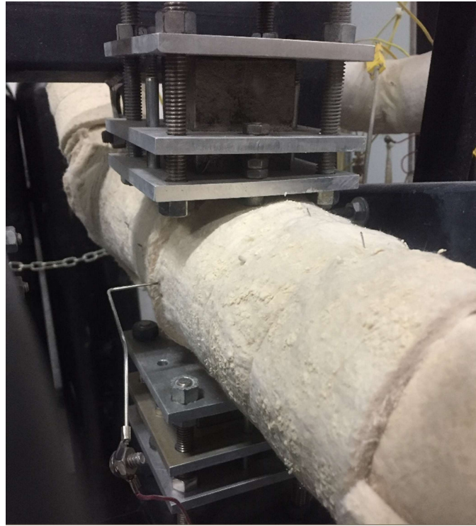
Figure 4-3: Photo of the PMIP-EMFM used for primary flowrate measurements.
