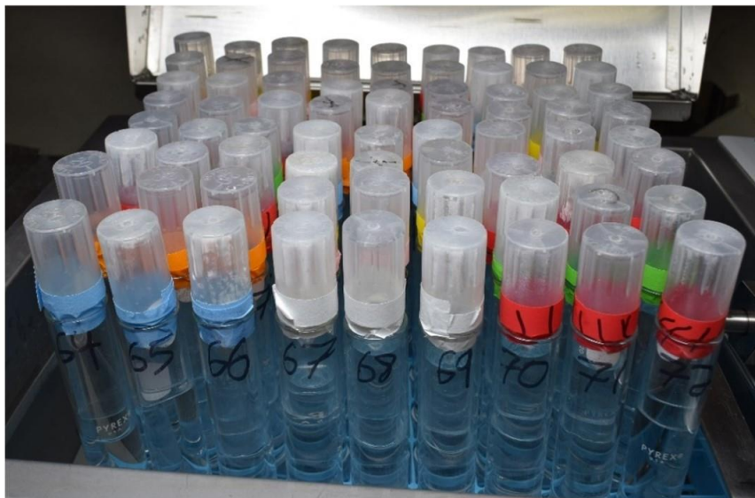
Figure A1: Water bath setup with the maximum 72 tubes and color-coded "insulating caps" that were used to help keep the whole-leaf sample up to temperature (50°C) and keep it completely submerged underwater inside the large test tube and under the bathwater surface.
