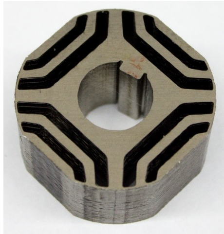
Figure 8-13. Manufactured SyR rotor section with integrated rotor key shifted to achieve an offset angle, \alpha = 57.5^\circ
