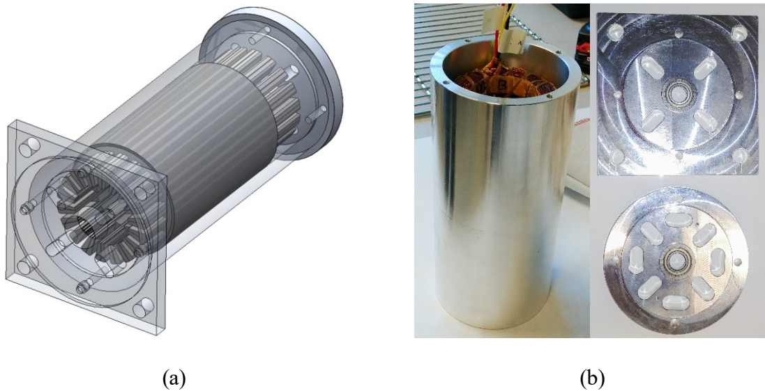
Figure 8-7. Housing and endplate design (a) CAD model showing stator, housing assembly (b) Manufactured housing and endplates.
