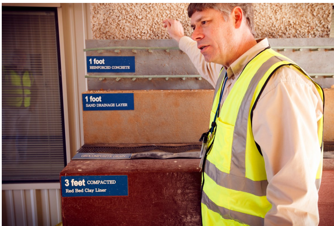
Figure 3.1. Top panel: Typical lower layer cross-section for LLW disposal facilities. (Modified from Powell et al. 2011). Lower panel: Rodney A. Baltzer, president of Waste Control Specialists, with a model of the installed barrier system at the Andrews, TX LLW facility (Stravato 2014).
