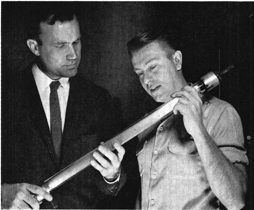
K. B. McAfee (left) and H. Kraft of Bell Telephone Laboratories are examining a cell which was built to study the separation of helium from gaseous mixtures. This cell contains roughly 1½ miles of 15-mil diameter glass tubing.
