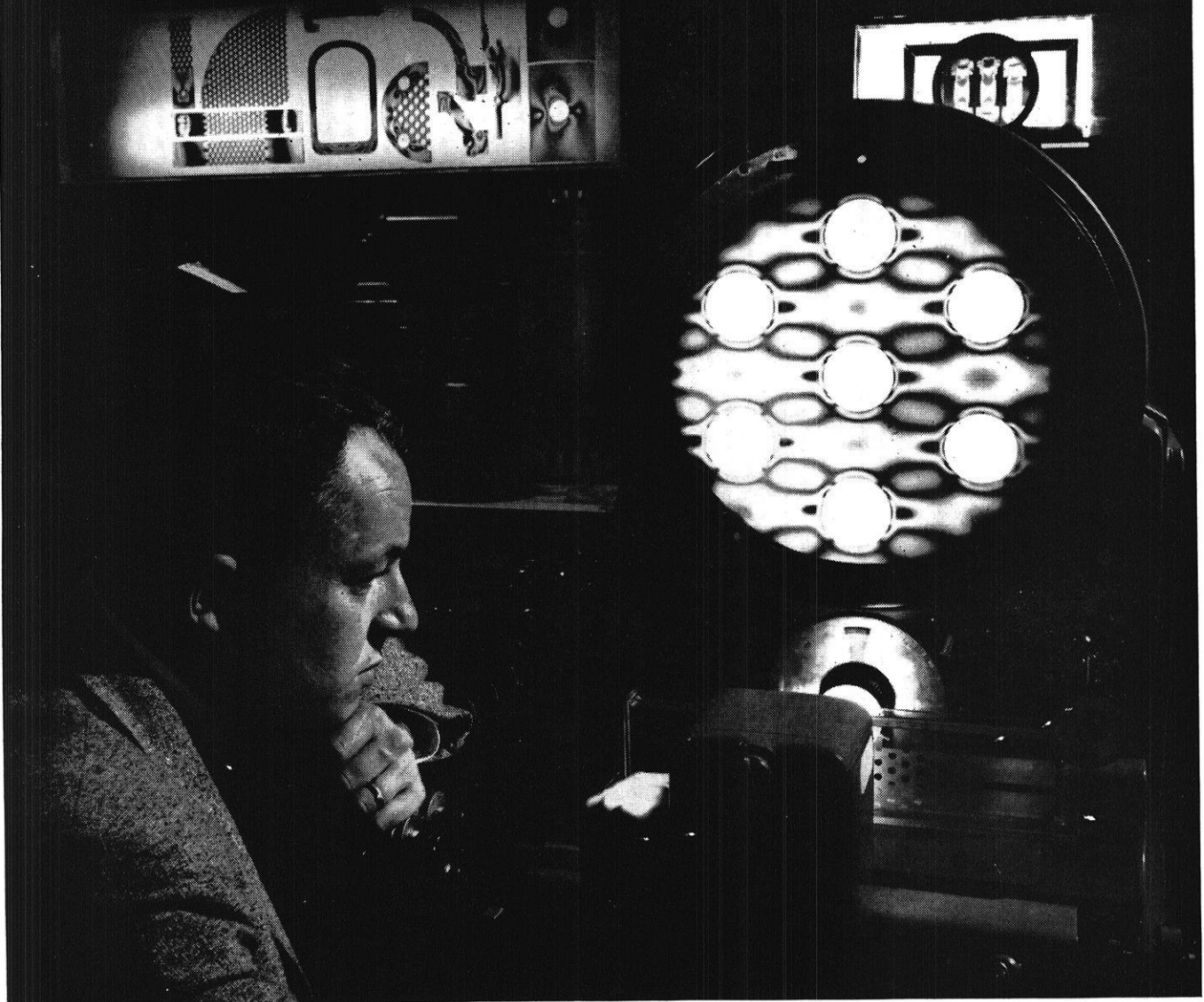
Westinghouse scientist Robert Sampson analyzes a special photoelastic model under polarized light to calculate the stresses which would be built up in an atomic reactor component now in the design stage.
