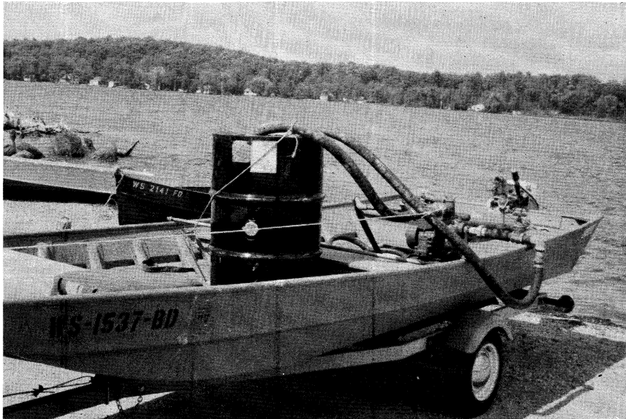
Chemical Spraying Equipment used in Weed, Algae, and Swimmers' Itch Control Program.
