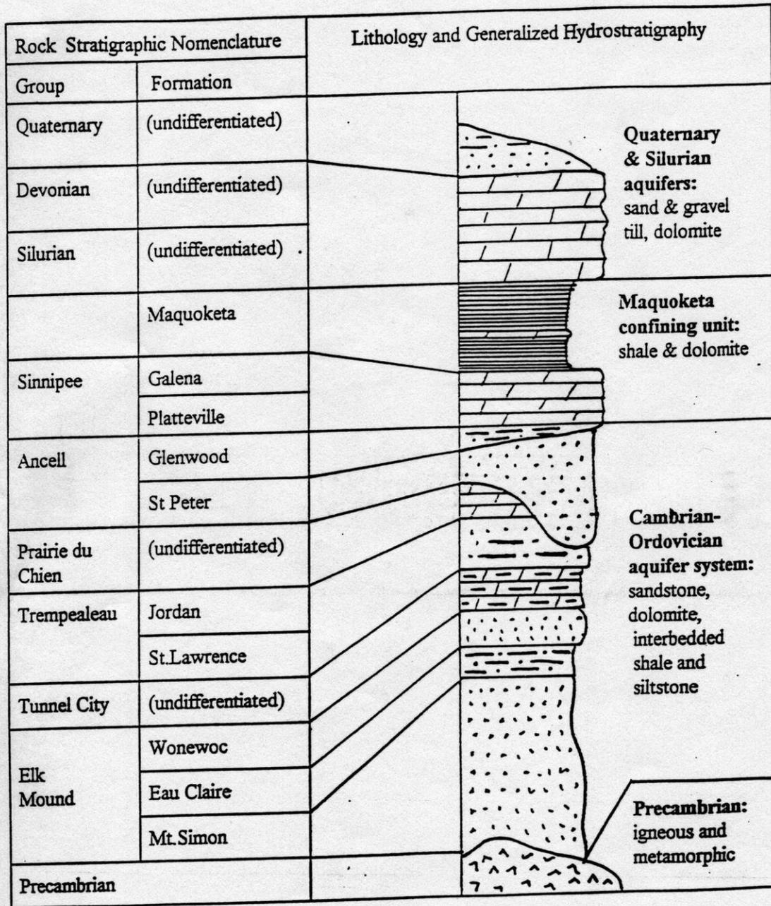
Figure 5. Regional hydrostratigraphy, adapted from Eaton et al, 1999.
