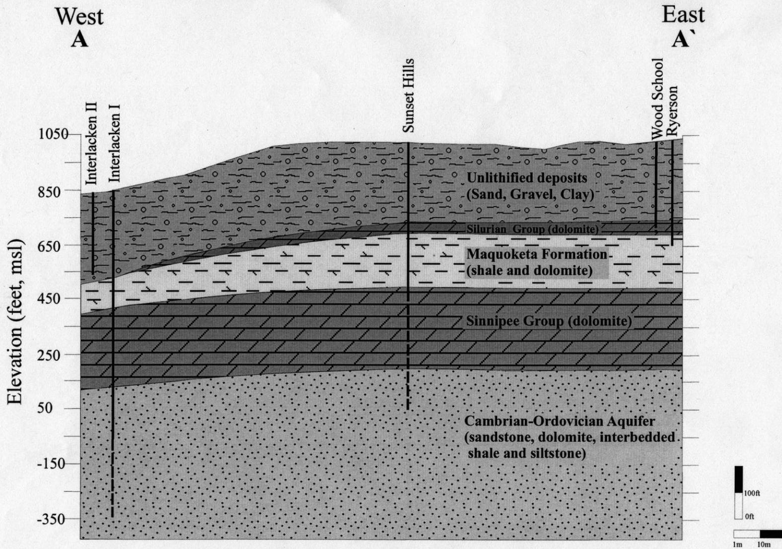
Figure 3. Geologic Cross Section
