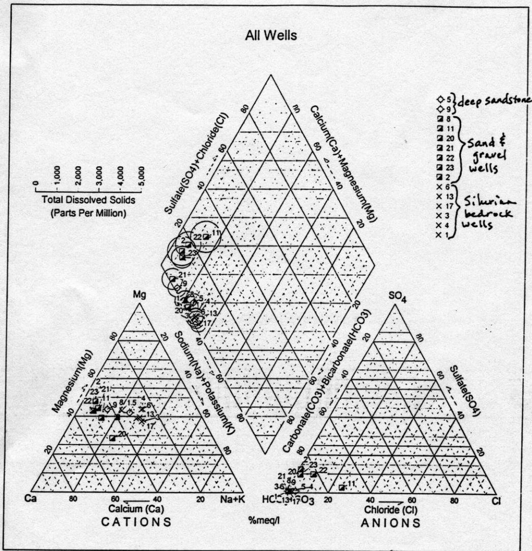
**Figure 6. Trilinear diagram of groundwater quality.**
