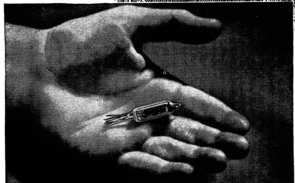
Typical Sylvania subminiature tube 1\frac{1}{4} " long, pencil thin—heart of vital electronic equipment.
